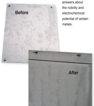
In most environments and applications, FreedomGray Satin T-Z Alloy™ will not stain other materials below them. However, drip edges and overhangs should still be designed to minimize water staining.
